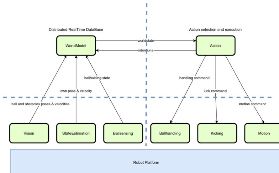
Fig. 3. Soccer Robot Architecture (Source: Eric Dortmans, Fontys)
